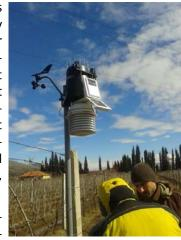
Three weather stations (Vantage Pro2, Davis Instruments) were installed at three different loca-
